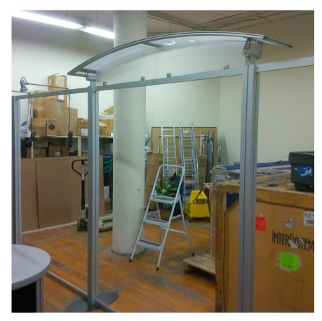
The frameworks are designed for easy assembly and teardo wn. Electrical strips will be mounted via velcro to the back side of the vertical posts, with markings for location. T he "wings" and posts, and their associated hardware fit into place and are held fast by adjustable tension hardware that is durable and easy to set up. Overhead lights clamp on to the horizontal posts above the graphics. The 3d Vitzrocell logo will hang in front of The plexiglass above the central graphic.
