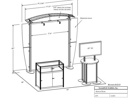
The sturdy metal framework is open, and will be used to display graphic backgrounds hung from the horizontal sections with velcro, and lightly stretched to reduce wrinkles and appear more "solid". The graphics will be illuminated from above.
